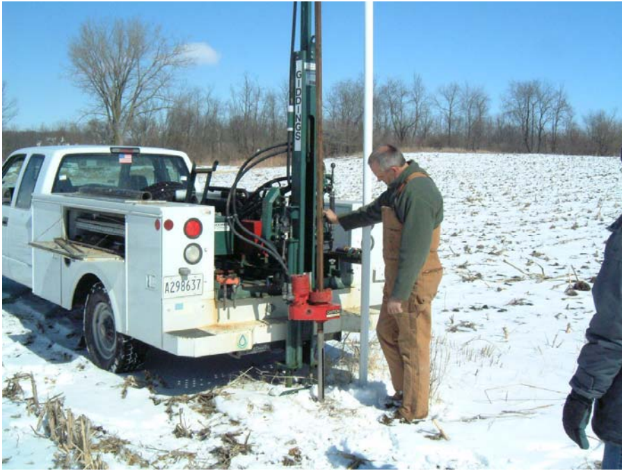
Figure 15. Roger Windhorn, Soil Scientist with the NRCS, conducts intensive soil sampling at the tile/wetland experimental sites to better understand the behavior of nitrogen and water at the site.
